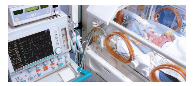
The STEPHANIE and SOPHIE NIV ventilation systems allows the nCPAP, nIPPV and synchronised nIPPV (SnIPPV) ventilation therapies, with or without backup ventilation, to be combined with EasyFlow system accessories.
